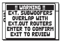
informs that one or more voice outputs have been addressed to MAIN outputs already configured for use with sub-woofer (see section 9.9). These outputs are also shown on the display area in the screen showing the total outputs. If two dot lines are displayed, this indicates that one or more overlaps are present:
