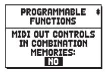
To switch off the light of MIDI stops when the Cancel piston is pressed (this screen is available only in models that allow to transmit MIDI codes).
