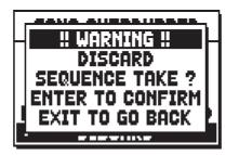
Warning you that the overdubbing will be lost. Press [ENTER] to continue – and therefore discard the recording – or [EXIT] to return to the previous screen.
