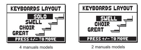
The display shows graphically the organ manuals with, next to them, the corresponding organ section when the Keyboards Inversion function is active. Using the [FIELD  $\blacktriangle$ ] and [FIELD  $\blacktriangledown$ ] buttons it is possible to move the cursor and position it in correspondence with the manual to be associated with the section, using the [VALUE +] and [VALUE -] buttons.
