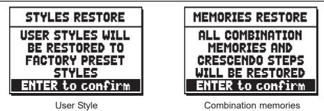
Press [ENTER] again to start the process or [EXIT] to abort it. When the process is complete, the following message will show:
