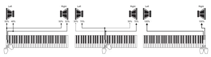
**DOUBLE CUSP**: there are two separate cusps, both resembling to the single cusp described above. The lowest keys sound in an intermediate position, between the centre and the outside, alternating (one on the right cusp, one on the left cusp). As the pitch rises, rises the signal is gradually distributed further and further to the outside, alternating.
