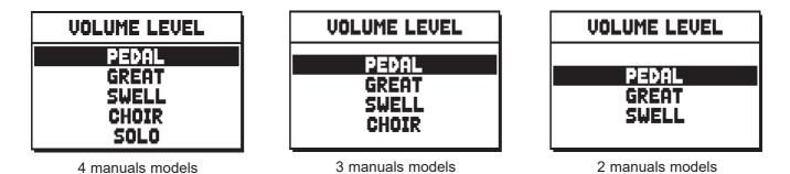
As usual, use the [FIELD  $\blacktriangle$ ] and [FIELD  $\checkmark$ ] and [ENTER] buttons to select the field on the display. Another way of displaying and adjusting the volume immediately is to hold out the draw-stop (NOT in models with electromechanical draw-stops) or hold down the rocker tab for a few moments in the voice on position, while the cursor is on the VOLUME LEVEL field in the VOICES menu, or in the function itself.
