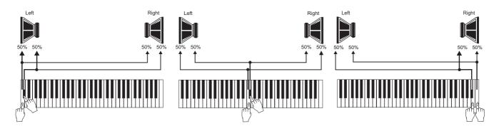
**POLY** ALTERNATING POLIPHONIC: the notes are distribute among the audio channels, so as to avoid having more unison frequencies on the same speaker. This limits the electrical sum of the signal, so as to favour the "in air" melting of the sound, as in a real pipe organ.
