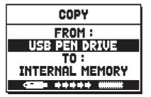
Now select the memory unit (**FROM** field), which contains the file to copy (from now on named "source") and the unit memory you wish to save the file in (**TO** field, called from now on "destination"). Once again, the available memories are an external flash drive ("USB PEN DRIVE" in the video page) or INTERNAL MEMORY. To select, use the [VALUE +] and [VALUE -] buttons.
