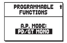
Select PD/GT MONO to activate the Monophonic Pedal function (with piston on). This function allows to play pedalboard registers on the Great. When doing this the pedalboard is deactivated and the stops become monophonic, with priority on the lowest note.
