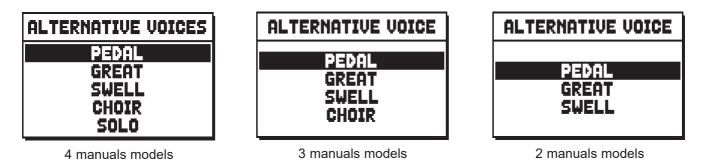
As for the other VOICES menu functions, the next step is to select the section of the organ containing the voice to be modified: this displays the list of the voices present in the chosen section.
