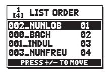
To move a piece into a different position, locate the cursor on the relative field of the file with the [FIELD  $\blacktriangle$ ] and [FIELD  $\blacktriangledown$ ] buttons and use [VALUE +] to move the position forward or [VALUE -] to set an earlier position. Finally, press [ENTER] to save the list or [EXIT] to return to the previous video page.
