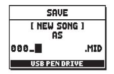
When composing the name, use the [FIELD  $\blacktriangle$ ] and [FIELD  $\blacktriangledown$ ] buttons to move the cursor and [VALUE +] and [VALUE -] to select the character. The first three characters can only be numbers, since they are required for future expansions of the instrument.
