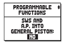
to turn off the All Swells to Swell and the Automatic Pedal when the Cancel piston is pressed:
