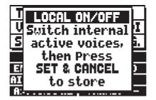
To set a voice in Local Off mode, operate its draw-stop or rocker switch so that its light goes out. After setting the setup required, press [S] and [C] together to save it. Accessing the Local Off setting function after this will trigger display of the status of the stops as follows:
