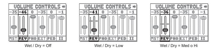
The **EXT SUB** parameter adjusts the level of the reverb effect in the signal on the output [GEN. SUB] and in the MAIN outputs eventually set as EXT. SUB (for more information see section 9.9).
