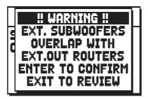
indicates that one or more MAIN outputs set for use with sub-woofer were previously assigned to one or more items using the EXT OUT ROUTERS function (see section 9.10). By pressing [ENTER] the voices assigned to the outputs affected by this overlap will therefore no longer be audible except with the sub-woofer(s) and therefore it is advisable to check and/or modify the assignment on the MAIN outputs via the EXT OUT ROUTERS function.
