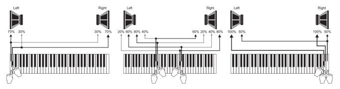
**DOUBLE WING**: the highest notes sound in the centre. As the pitch lowers, the signal is gradually distributed further and further to the outside, alternating.
