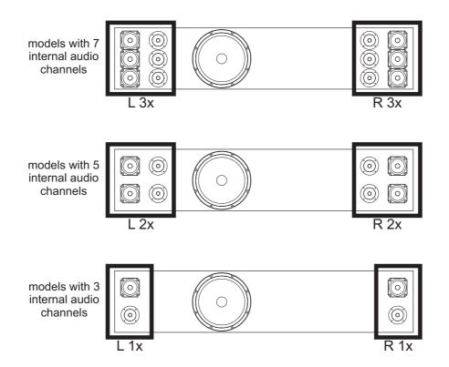
Arranging the voices in the two channels simulates the position of the windchests of real pipe organs, since they were usually placed in different areas. It also simulates the different position of the pipes inside the windchest, which could vary according to the stop played, the period when the organ was built and the wishes of the builder.
