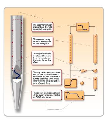
incorporating the principal physical parameters ie. construction geometry, materials used, and pertaining air pressure, etc.
