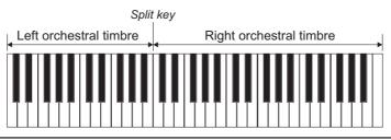
**Layer**: two stops (named 1 and 2) overlapped along the whole manual / pedalboard. This kind of voice is shown as the names of the two stops with a "+" in between.
