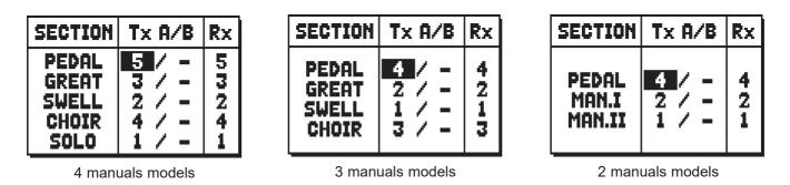
The **SECTION** column lists the organ sections; for each section a channel from the Tx A/B and Rx can be assigned. Press [EXIT] to leave the screen and save the settings.
