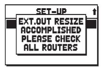
The repositioning takes place through several adjustments, so as to use the outputs as already configured before. However, some routers might be placed differently from what you intended. Therefore, at the end of the procedure, the system will advice to check again the settings through the EXTERNAL OUT ROUTER function.
