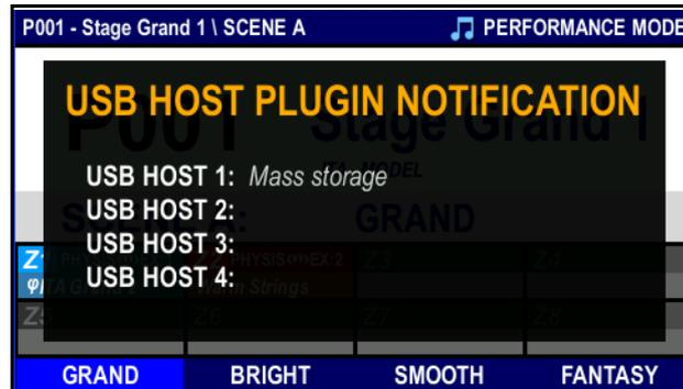
The message indicates the name of the USB device and the [USB HOST] connector in which it was inserted. Now wait a few seconds for the message to disappear, then press the [SYSTEM] button on the front panel in the section named MODE. The display shows the first page of the SYSTEM menu:
