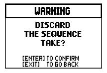
Warning you that the overdubbing will be lost. Press [ENTER] to continue – and therefore discard the recording – or [EXIT] to return to the previous screen.
