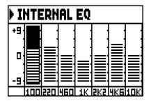
In the lower part of the screen there are the seven central band frequencies. To move the cursor from one band to the other, use the buttons [FIELD  $\blacktriangle$ ] e [FIELD  $\blacktriangledown$ ].
