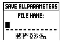
where it is possible to give a name to the saved file. To select the characters, use the buttons [VALUE +] and [VALUE -], to move the cursor use the buttons [FIELD ▲] and [FIELD ▼]. When the name is complete, press [ENTER] to save the file.
