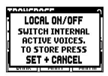
To set a voice in Local Off mode, operate its draw-stop or rocker switch so that its light goes out.
