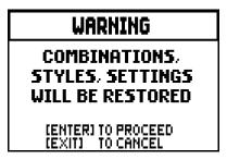
Press [ENTER] again to start the process or [EXIT] to abort it. When the process is complete, the "FACTORY SETTINGS SUCCESFULLY RECALLED" message will appear.
