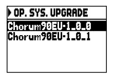
use the [FIELD ▲] and [FIELD ▼] buttons to select the file you wish to install, then press [ENTER]. The system informs you that the currently running operating system will be replaced with the version on your USB drive.
