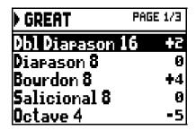
During the edit the stop will be on and can be played for better, quicker adjustment. Other stops can also be switched on to assess the overall effect of the changes. To quit the function and save the values press [EXIT]. The changes made will be automatically saved in the current organ style.
