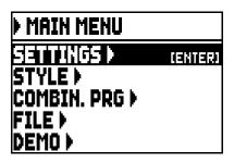
As in the main video page the cursor is represented by the field with inverted colours. To move it, press the buttons [FIELD  $\blacktriangle$ ] and [FIELD  $\blacktriangledown$ ].
